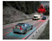
**Oncoming Mitigation by Braking** A Volvo Cars safety world first, this innovation can detect vehicles heading towards you on the wrong side of the road. If a collision can't be avoided, it will brake your car automatically to help reduce the effect of a collision.
