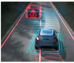
Oncoming Lane Mitigation Using automatic steering assistance, this system helps you avoid collisions with oncoming vehicles. If you drift across the lane markings in the way of an oncoming
