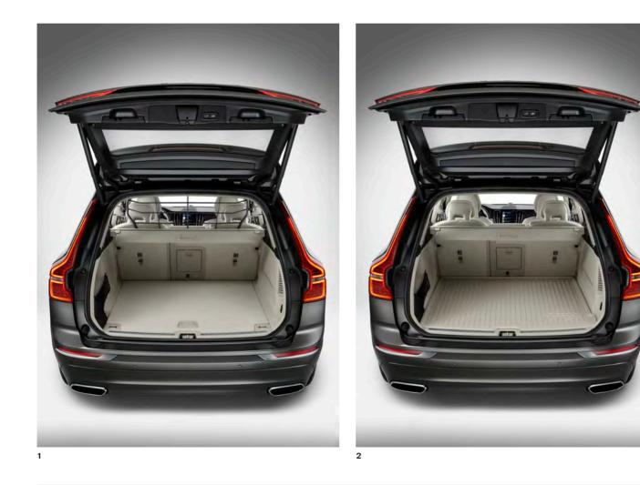
1. Protective steel grille. 2. Load compartment mat, plastic.
