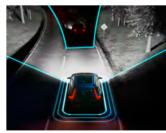
Full-LED Active High Beam illumination Full-LED Active High Beam illumination To give you the best view, our Full-LED head-lights allow you to drive with high beam on all the time, without dazzling others. It detects road users ahead of you and automatically shades the part of the high beam that would dazzle them.
