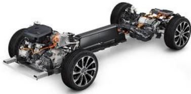
The way we've designed the T8 Twin Engine gives you more than just efficiency – you will notice how well balanced and responsive the car feels on the road, and how quickly it reacts to changes of direction. By mounting the electric motor over the rear axle and fitting the battery along the car's centreline, we've given the S90 with near-perfect weight distribution, a key element in creating agile handling.
